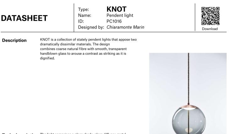
**Tech. description** The light comprises a glass shade, glass diffuser, metal component with LED module, and linen rope and is suspended from the ceiling canopy with a special bracket. The bottom section of the light is engineered as SELV.
